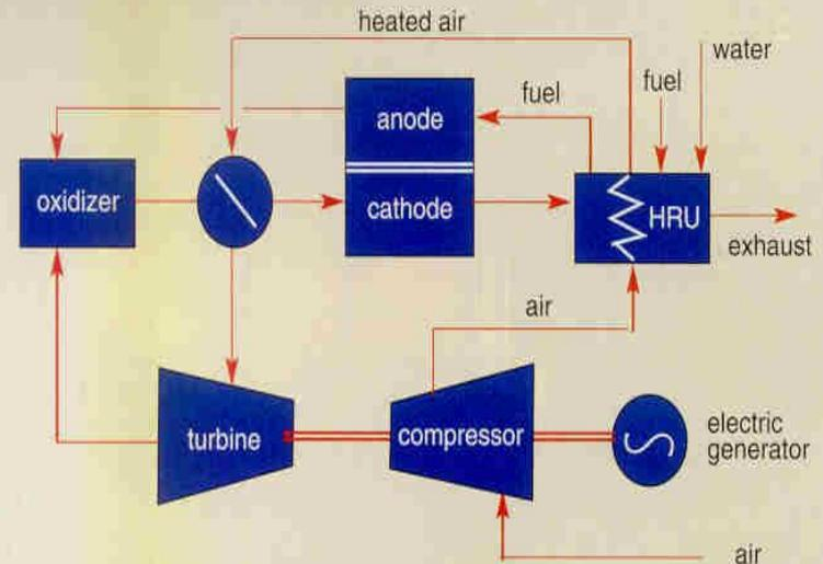
Coal or biomass is gasified to  $H_2$  and  $CO$  and fed to HRU. Compressed air is heated by HRU, expanded thru gas turbine, and then used as fuel cell oxidant. Cathode exhaust is used to fuel preheat and water vaporization. Anode exhaust is used for cathode air preheat.
