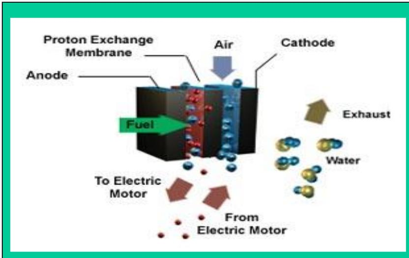
PEM fuel cell uses a polymer membrane as its electrolyte, contains water, operates up to 100 C, low tolerance to CO. Can be started quickly, good for peak and emergency power, slightly lower efficiency than PAFCs.
