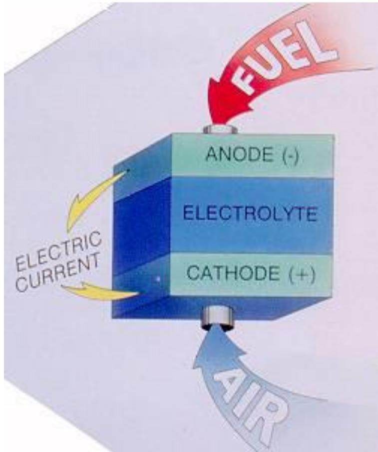
**Fuel Cell:** an electrochemical device, closely related to the battery, that can generate electricity from hydrogen, which in turn can be extracted from natural gas or other hydrocarbon gases through a chemical process called reforming.
