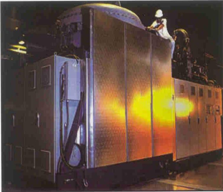
**Tubular solid oxide hybrid.** This 225-kW hybrid system on test at the University of California is designed around Siemens Westinghouse fuel cells and Ingersoll Rand microturbine which runs off the 850 C exhaust temperature of the fuel cell module.
