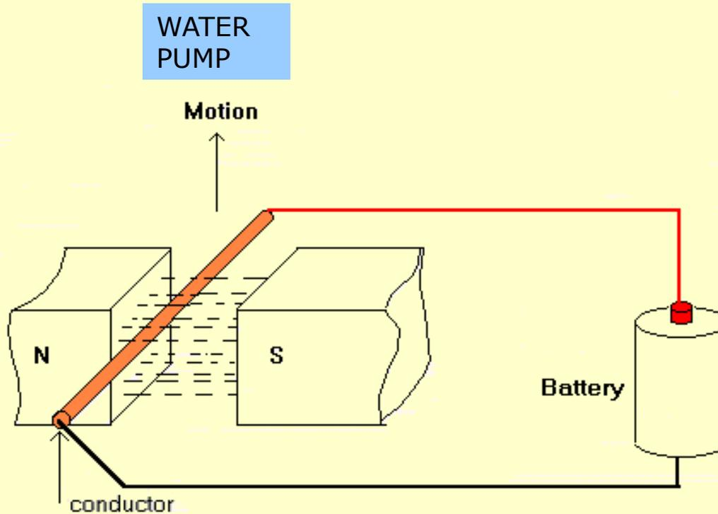
Current from battery or electrical supply cuts the magnetic field resulting in a force that drives or rotates the water pump to do work.
