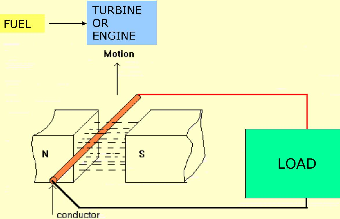
The fuel is burned and its energy is captured to drive a turbine or a piston engine which moves a coil against a magnetic field, causing a current to flow and supply power to a load.
