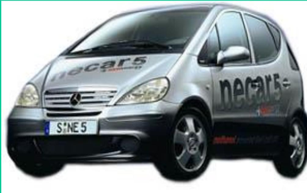
Daimler-Chrysler rolled out last November 2000 the fuel cell car - NECAR 5; peak velocity of 150 kph; 450 km per one tank of hydrogen fuel.
