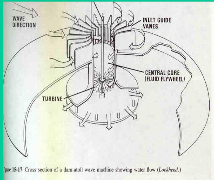
Figure 15-17 Cross section of a dam-atoll wave machine showing water flow (Lockheed.)
