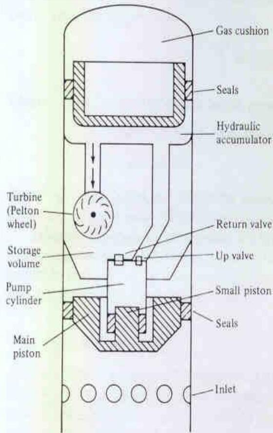
Figure 15-14 Schematic of a hydraulic-accumulator wave machine [151].
