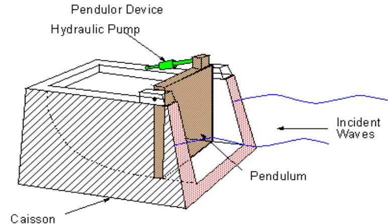
Pendulor device is a rectangular box which is open to the sea at one end; pendulum flap is hinged over this opening so that it swings back and forth to power a hydraulic pump and generator.
