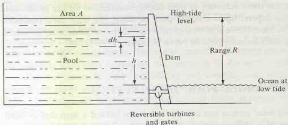
Figure 15-21 Level changes during power production in a single-pool tidal system.
