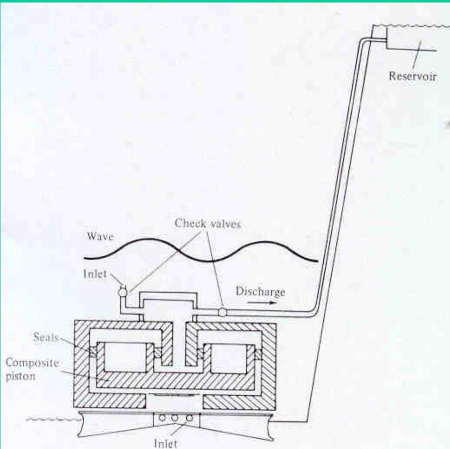
Figure 15-15 Schematic of a high-level reservoir wave machine.
