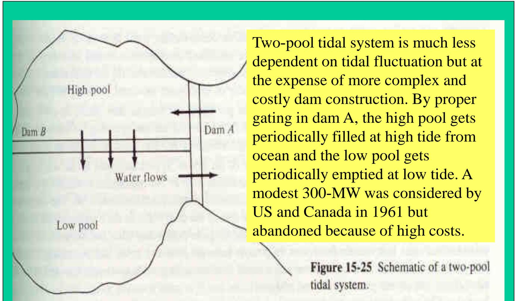
Two-pool tidal system is much less dependent on tidal fluctuation but at the expense of more complex and costly dam construction. By proper gating in dam A, the high pool gets periodically filled at high tide from ocean and the low pool gets periodically emptied at low tide. A modest 300-MW was considered by US and Canada in 1961 but abandoned because of high costs.
