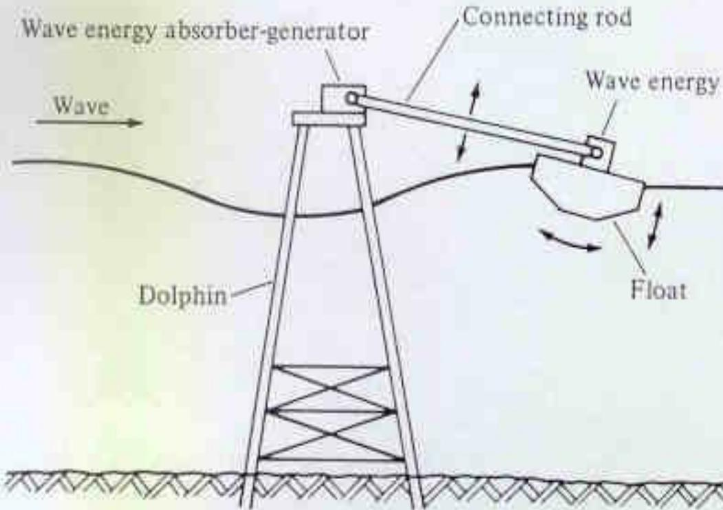
Figure 15-16 Schematic of the dolphin-type water generator (U.S. RESEARCH LABORATORIES)
