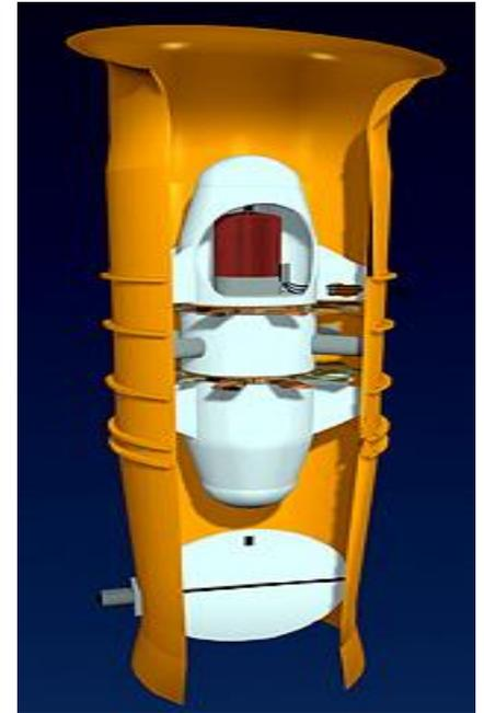
Wave energy collectors used in Limpet and Osprey modules are partially submerged shells into which seawater is free to enter and leave; water level rises or falls in sympathy; column of air above water level is alternately compressed and decompressed, generating a high velocity air going in and out of an exit blowhole; energy extracted thru a pneumatic (air) turbine.
