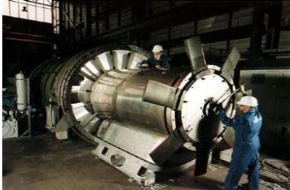
Prof. Alan Well's turbine (founder of Wavegen) has the unique property of turning in the same direction regardless of which way the air is flowing across the turbine blades, thus continue turning on both the rise and fall of wave levels within the collector chamber.
