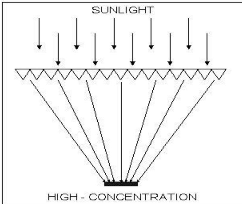
Solar cells become very inefficient when exposed to concentrated sunlight. EPRI thru Amonix solved the solar cell stabilization problem by developing **back-junction point-contact** silicon solar cell in 1989. Inexpensive flat plastic *Fresnel* magnifying lenses focus and concentrate sunlight 250 times onto a small expensive silicon cell. With tracking, 30% more energy is captured. Has possibly the lowest levelized cost (\$/kWh) of solar PVs.
