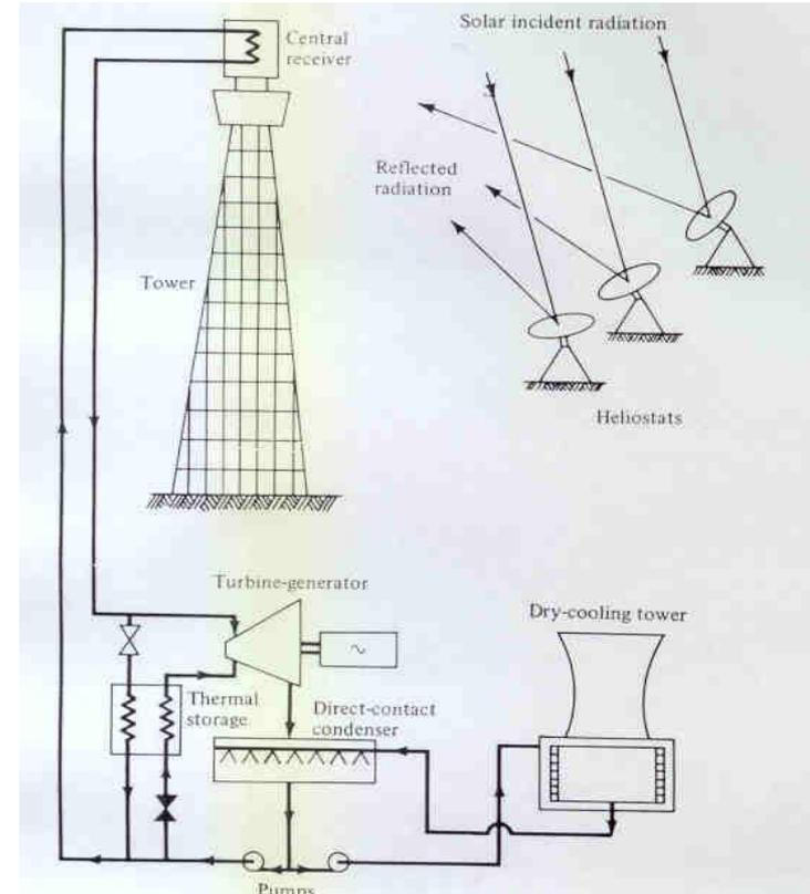
Solar-Thermal Central Receiver (Solar Tower)
