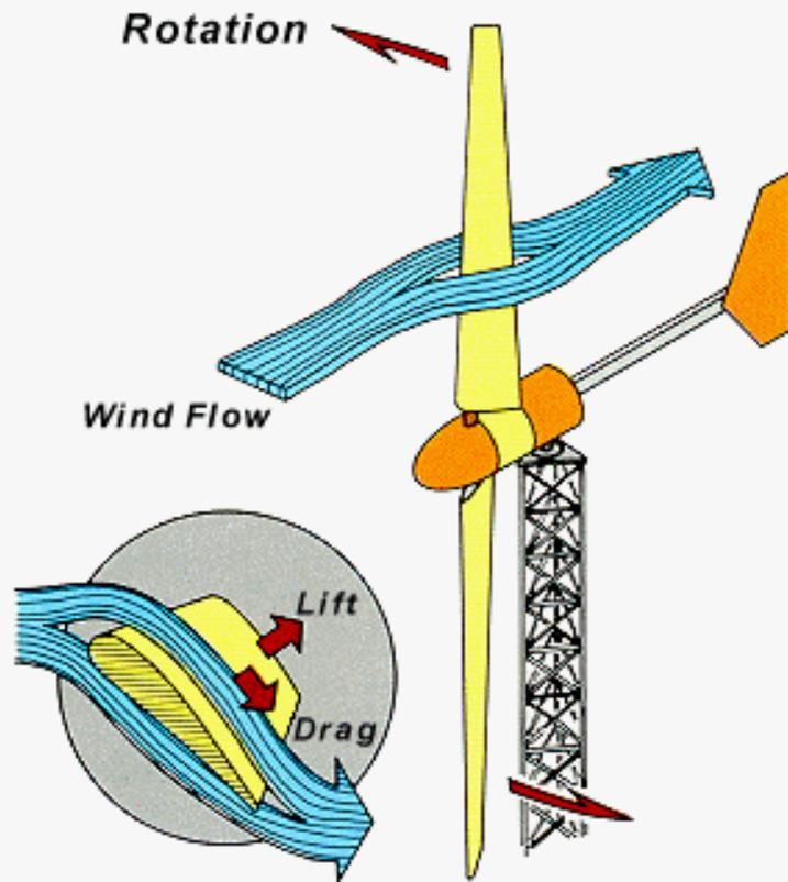
*Principles of Wind Turbine Aerodynamic Lift*
